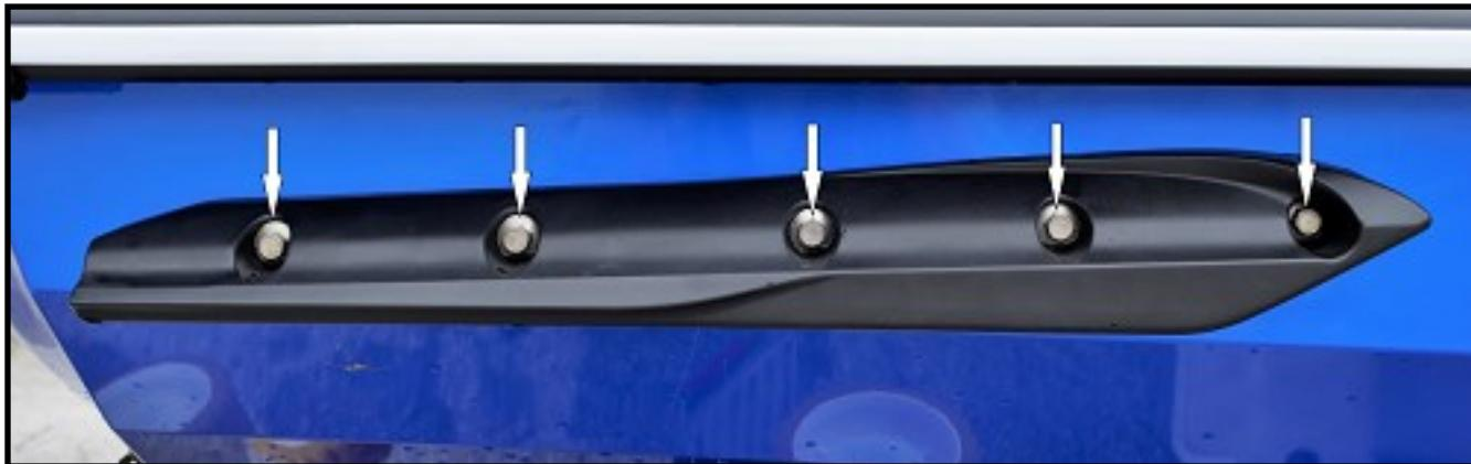
Place supplied backing plate (note L.H. and R.H. are different) on hull and secure with supplied 8 x 40 mm socket head cap screws and flat washers. **NOTE: Do not apply silicone or other sealer between hull and backing plate. Apply blue Loctite on screw threads. Torque screws to 11.8 ft•lb (16 N•m).**
