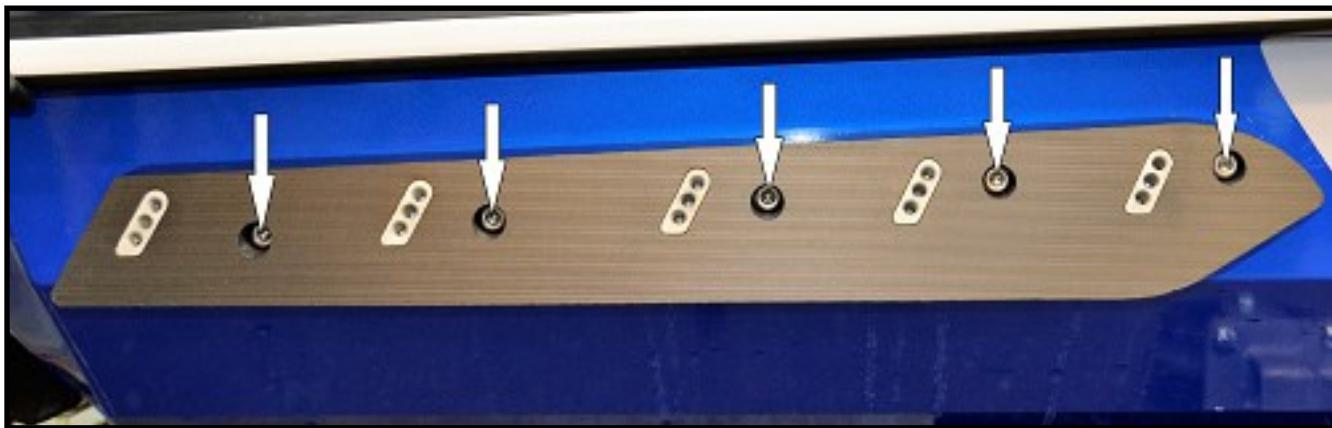
Place supplied 8mm wave washers on 8 x 25mm button head cap screw. Insert one bolt and washer combination through the center bolt location of sponson fin. Do not tighten. Repeat with the four remaining bolt and washer combinations. Be sure to put all bolts at the same height in the backing plate inserts. We recommend starting in the middle position. Tighten all bolts. **NOTE: Apply blue Loctite to bolt threads. Torque to 11.8 ft•lb (16 N•m).**
